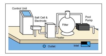
Once the cell is located, connect the black multi-core cable to the cell. The blue wire must be connected to the blue terminal. The cable is designed to come from below the cell. Make sure wing nuts are correctly tightened to ensure good contact.
